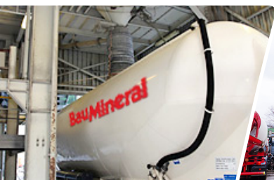
Fly ash collection at the power station
